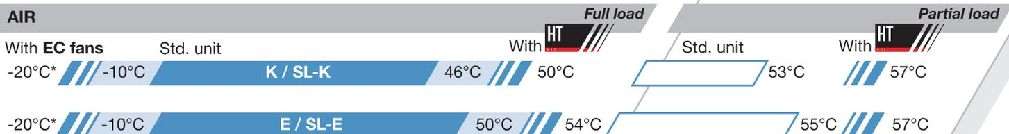
\*requires antifreeze and double insulation on heat exchanger, piping, pumps.
